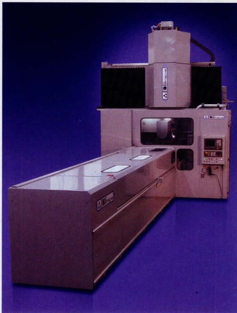
The smart workholding features employed on the Bertsche P5 bridge mill, which is designed for machining long parts, permits mill, drill, rout, saw-cut, and inspection operations in a single part setup.
