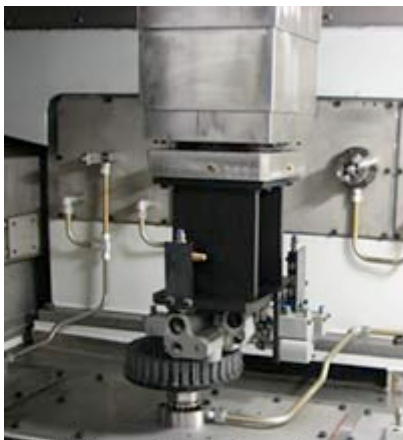
Hybrid design enables the iJet to do mechanical brush deburring and hole chamfering, as well as high-pressure water deburring.
