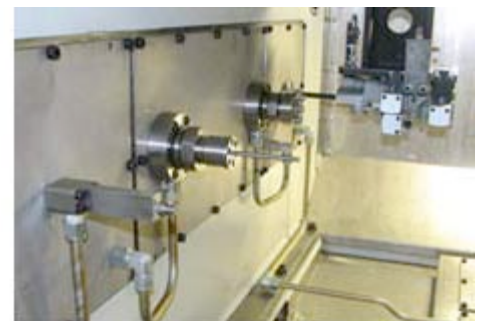
Horizontal stations on the iJet deburring system include a horizontal direct nozzle, rotary manifold, and 90° direct nozzle.
