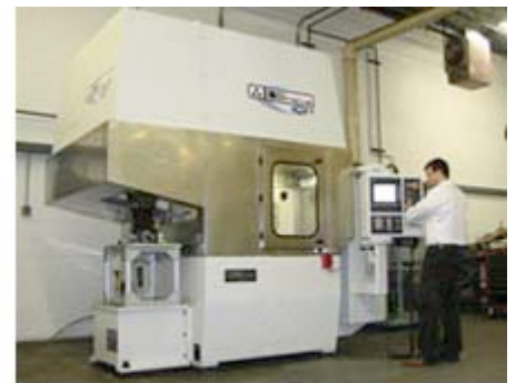
The Bertsche iJet CNC hybrid high-pressure waterjet deburring and washing center handles parts as large as 300 x 300 x 200 mm. It moves the part to the waterjet nozzle -- not the nozzle to the part, and generates water pressure to 10,000 psi (69 MPa).
